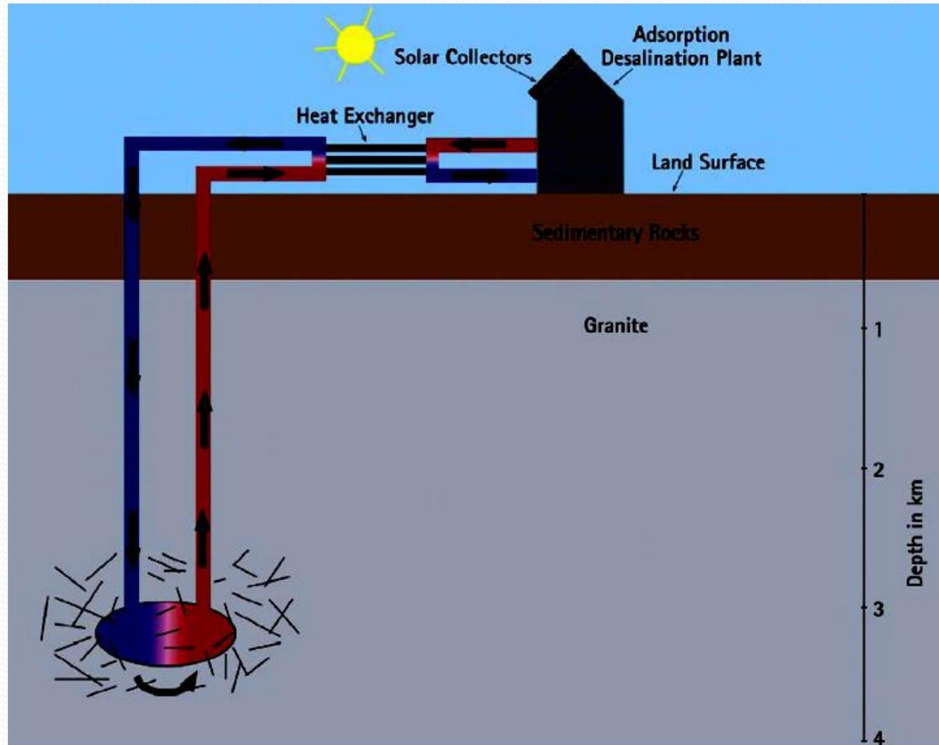
Schematic representation of a geothermal energy powered desalination plant
