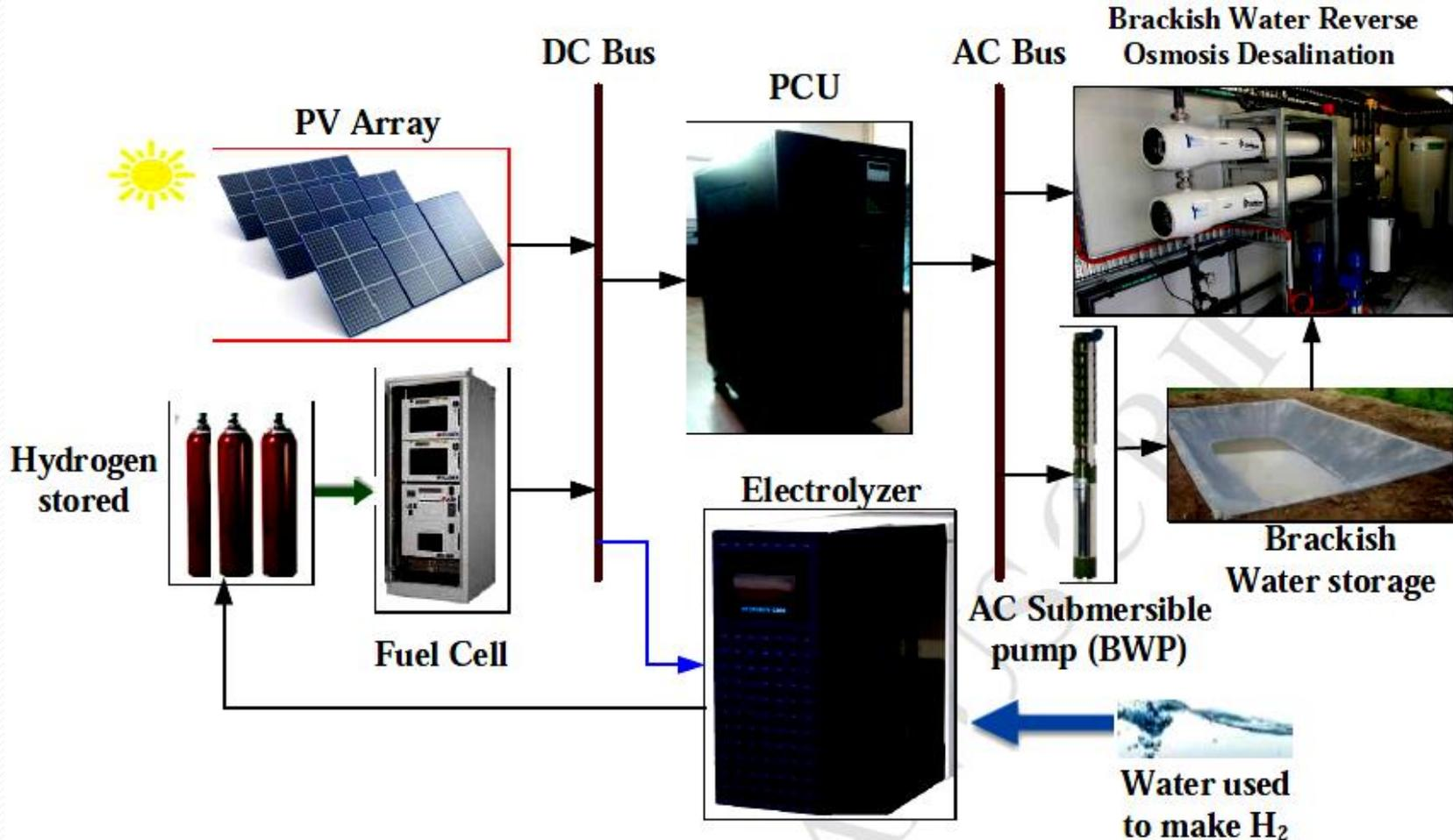
The system consists of PV array, self-charging fuel cell, electrolyzer, power conditioning unit (PCU) and hydrogen storage tank.
