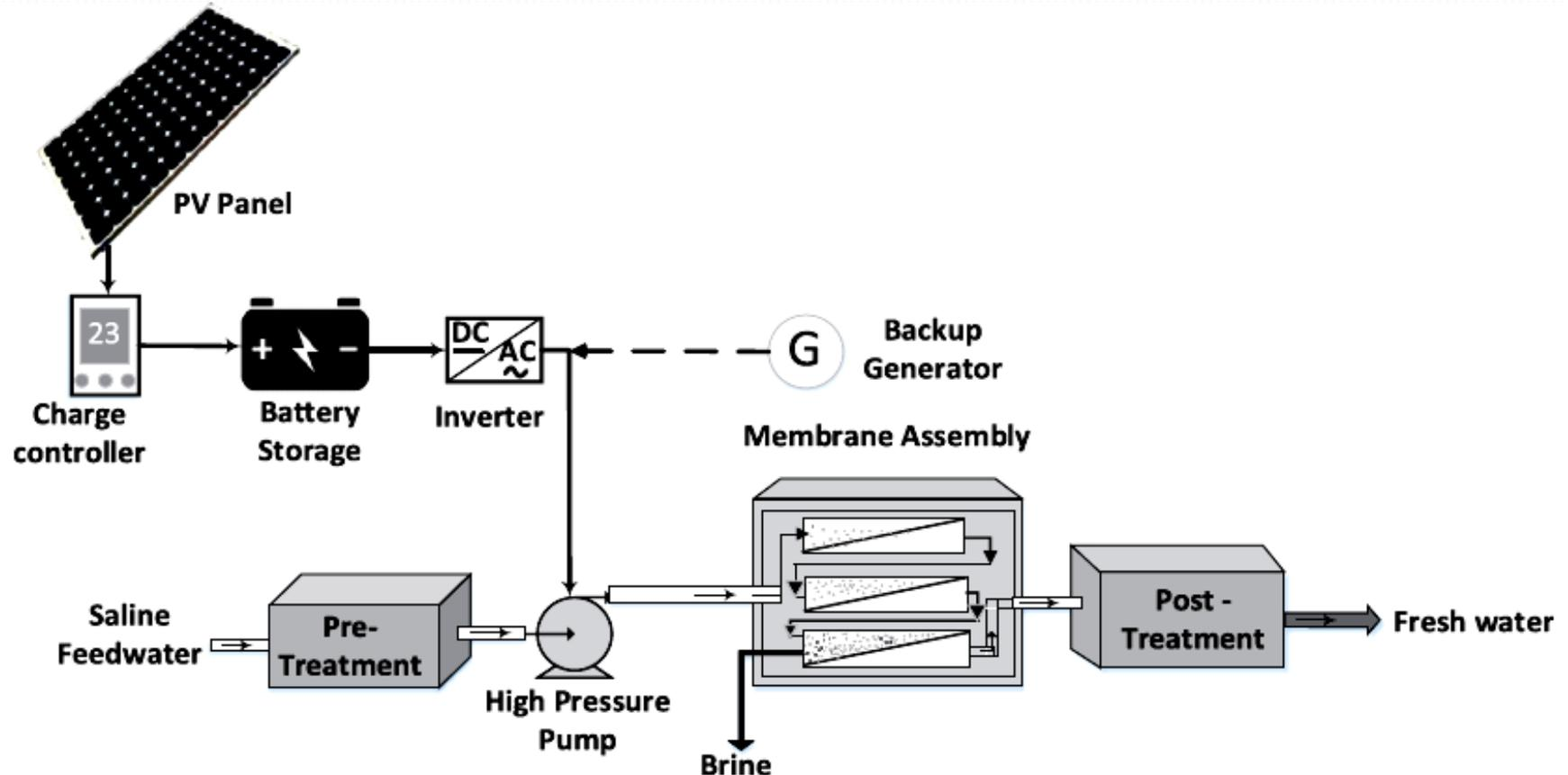
A schematic representation of a PV-RO system
