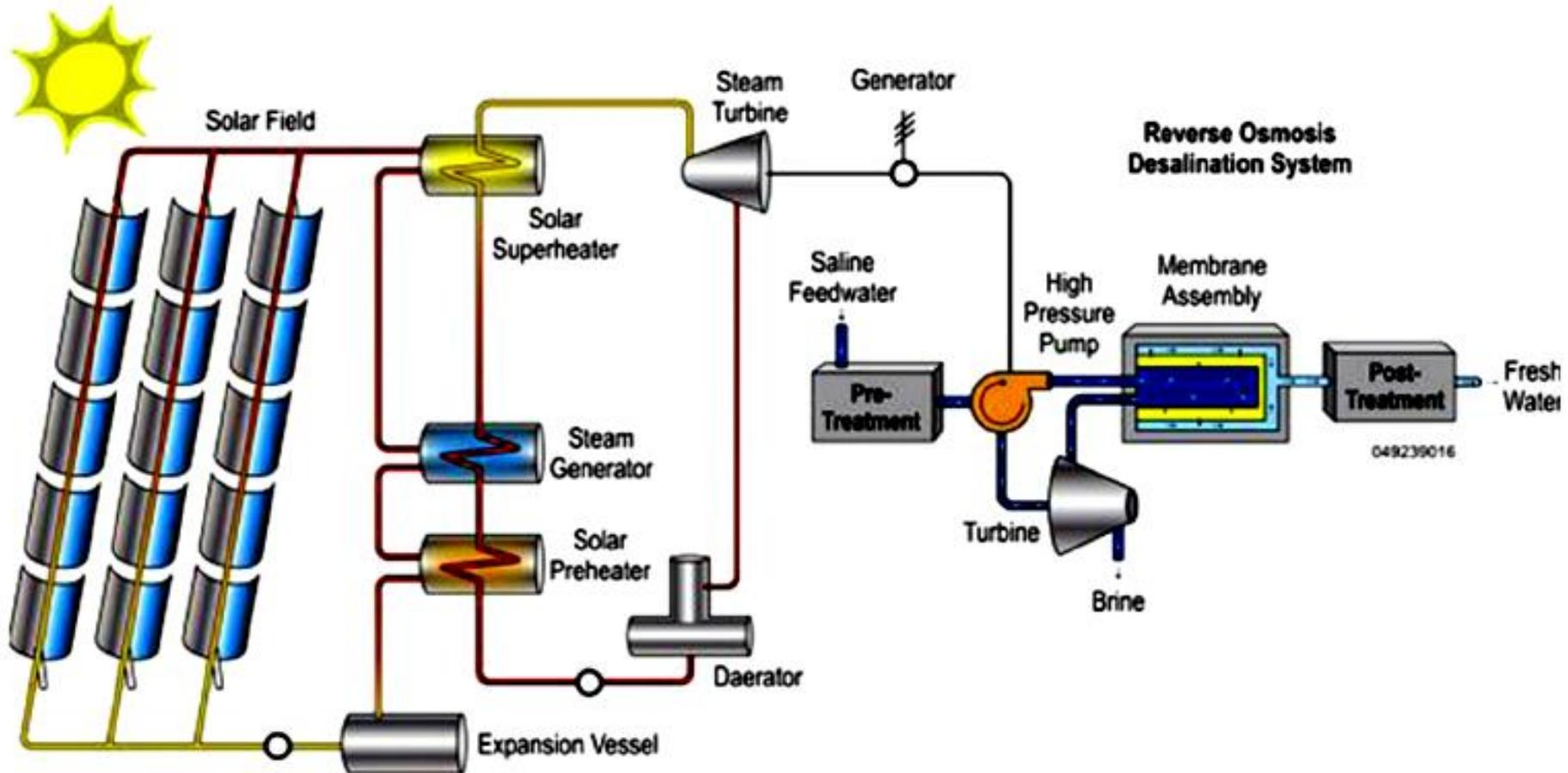
Schematic diagram shows the operating principals of Rankine RO unit with energy recovery
