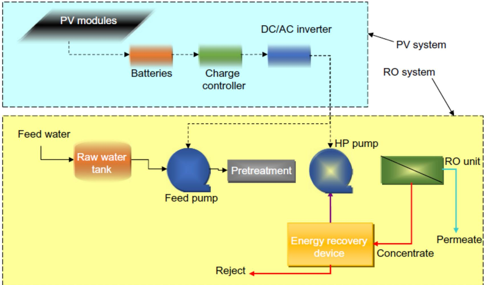
Basic design model of a RO water desalination system powered by PV.
