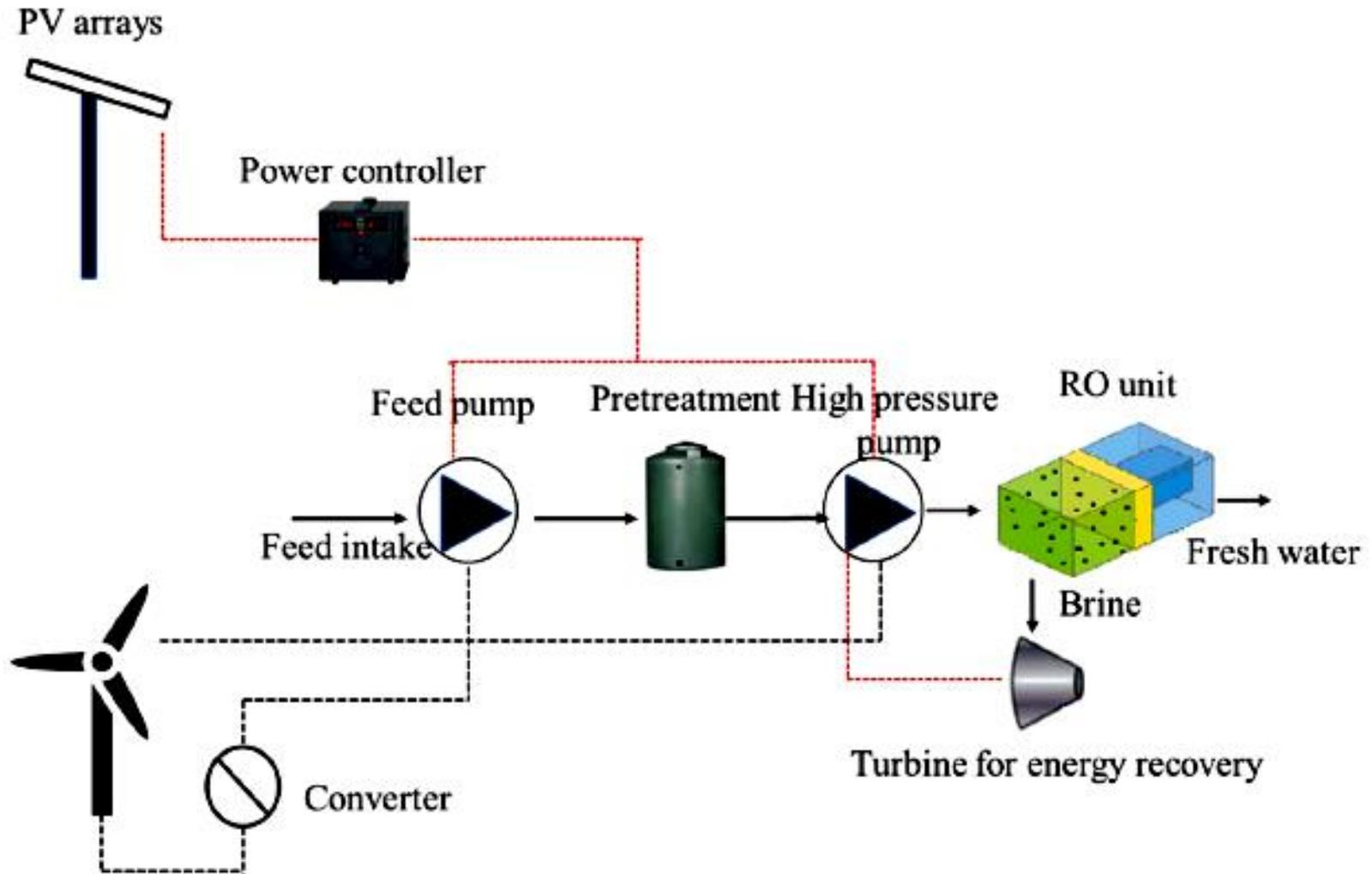
Schematic diagram of solar/wind driven RO system
