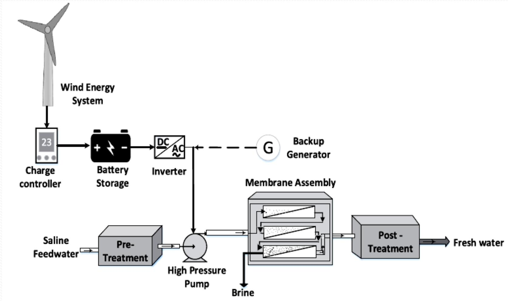
Schematic representation of a typical wind-RO desalination system
